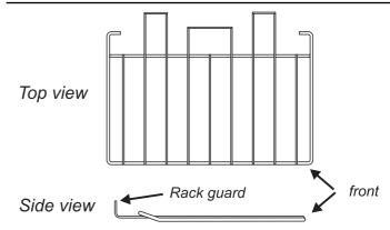
the rack guard should be at the back pointing upwards
